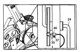
Turn the right crank arm for a moment. Repeat until the console displays correct feedback. When the reed switch is correctly adjusted, reattach the right side shield and the right pedal.
